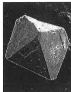
Figure 2b. SEM image of a cyclohexamantane crystal magnified 150x.
